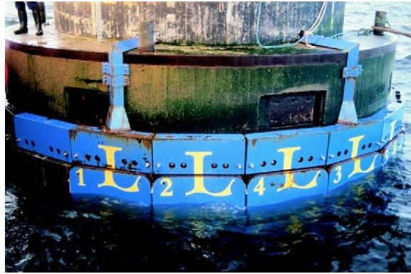
Figure 6-9 STRICE measurement panels: (a) schematic of panel numbering and orientation; (b) mounting configuration (Kärnä and Yan, 2006).
